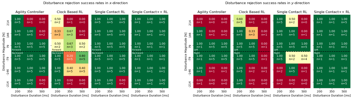
Fig. 3. Disturbance rejection success rates for various humanoid SaW controllers in the x -direction (left) and y -direction (right). Results show that our Single Contact reward function outperforms competing alternatives. * Results for Single Contact++ are incomplete due to the robot being damaged in unrelated experiments, noting that experiments for the largest forces were completed before attempting to fill in the rest of the table.
